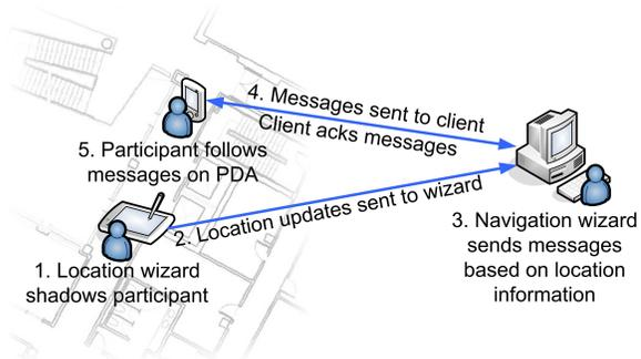
Figure 3: System interaction diagram. Location wizard provides location information on the participant ( $x$ ,  $y$ , floor, and orientation) (1) sent over wi-fi (2), while the navigation wizard uses that location information to decide which messages to send (3). Messages (to display images, text, and play audio) are sent to the client device over wi-fi and acknowledged for robustness (4). Participant then follows the direction or prompt displayed on device (5).
