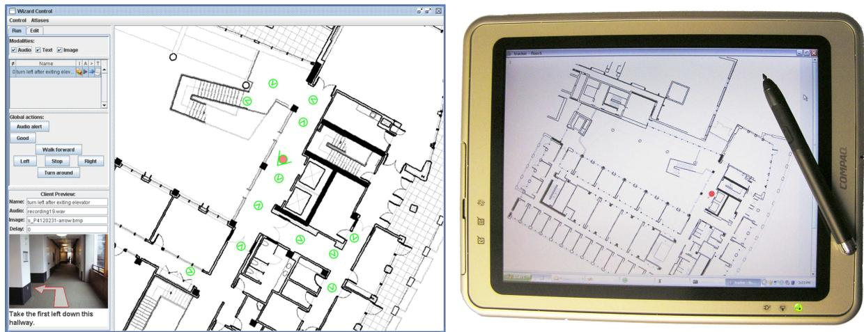
Figure 4: *Left*: Screen shot of the navigation wizard GUI running on a desktop. Green marks on the map show where pictures were taken from, and are used to send prompts to client. Solid red mark shows information from location wizard. *Right*: Location wizard GUI running on a tablet PC. Red mark shows participant location and orientation.
